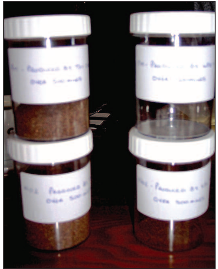
The two filled jars on the left contain emissions from an unconverted cab. The two almost empty ones are from the LPG cab
