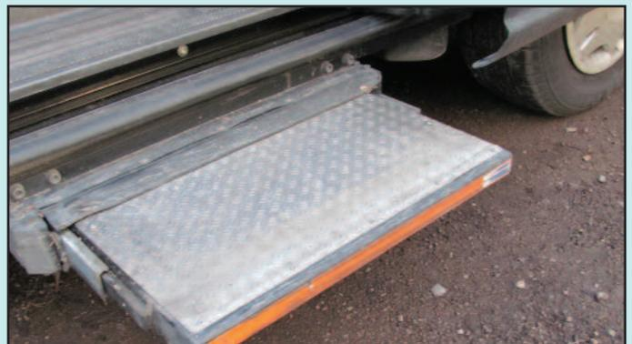
One final tip regarding the steps’ sliding mechanism - the runners should be lubricated with a silicone based spray several times a year to ensure their smooth operation.
