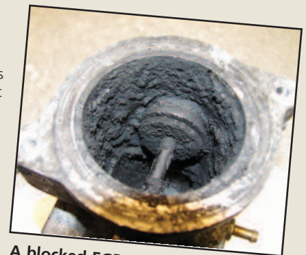
A blocked EGR valve can lead to lack of power and poor fuel economy among other things
