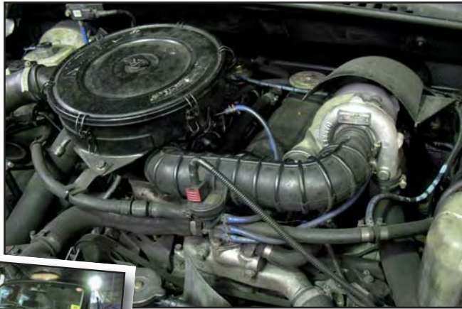
The TX1 Nissan engine looks normal except for the silver aluminium turbo housing and big black hose lying across the top. inset: The TX1 is on its way to Germany
