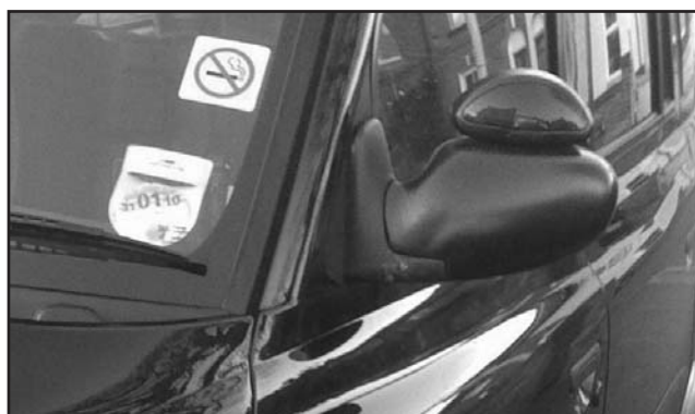
The Frog-eye attached to the normal taxi mirror
