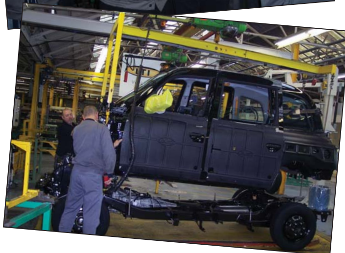
A TX4 body drops onto the chassis
